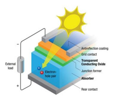
**Figure 2.** Schematic of a photovoltaic cell. Nanomaterials have the potential to enhance the performance of each layer in the cell - from more transparent coatings and more conductive electrodes to more efficient absorbers. Image credit: <a href="NREL">NREL</a>
